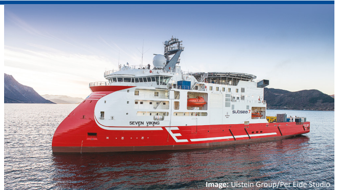
Image: Ulstein Group/Per Eide Studio The Ulstein X-BOW® hull is designed to improve handling in rough seas and to lower fuel consumption by causing less hydrodynamic drag
