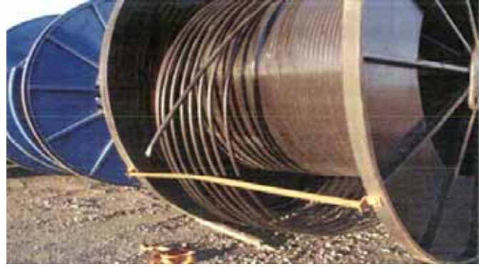
The unwound reel after the ratchet strap was removed and the stored energy released.
