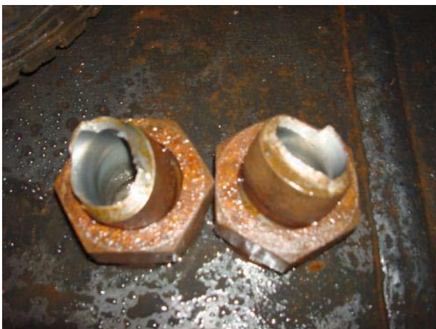
Figure: showing damage to couplings
