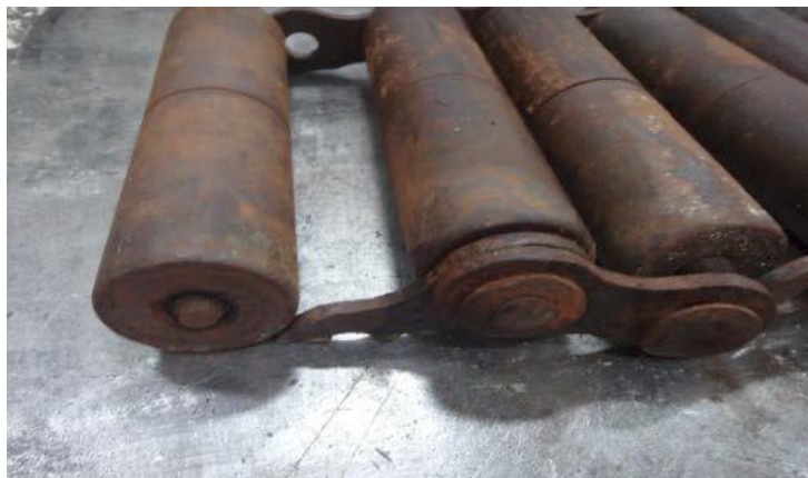
Figure: sheared '8' link plate
