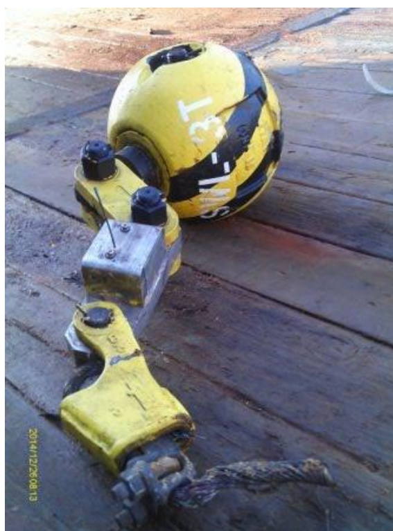
Figure: crane block that fell
