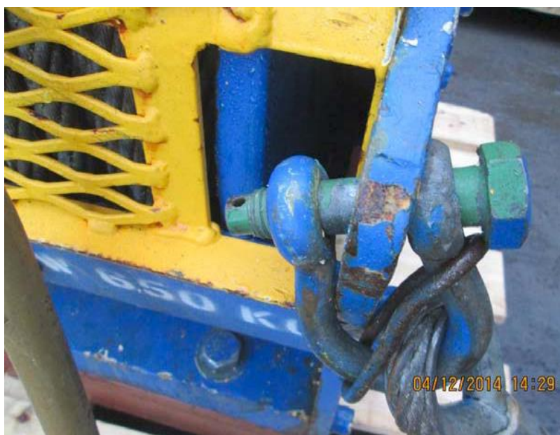
Figure: condition in which lifting equipment was left – showing missing nut and split pin
