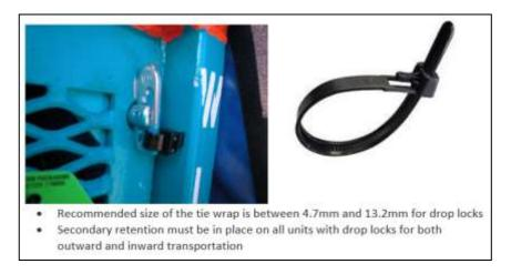
Unsuitable secondary retention methods include linchpins, R-clips, spring/roll/nappy pins or any other type of pin device. All these means of secondary retention for lifting equipment or securing at height can spring open or be knocked out.
