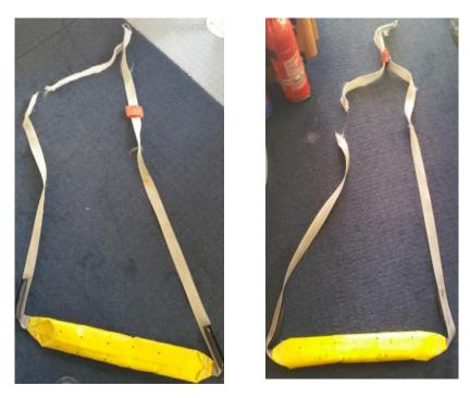
Figure: showing typical SB rescue slings
