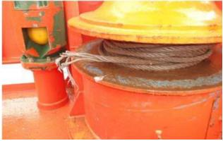
Figure: capstan showing parted wire
