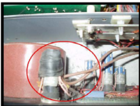
Unauthorised modification to electrical equipment
