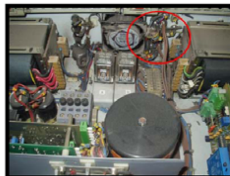
Unauthorised modification to electrical equipment
