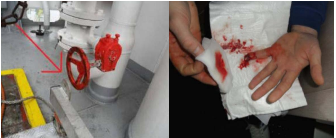
Showing pinch-point between gangway frame and valve, and injured finger
