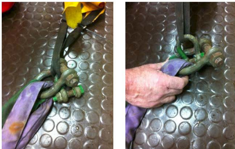
Showing arrangement of shackles that allowed lift bag to come free and ascend to surface
