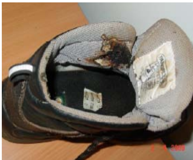
Figure 2 – Injured person's safety shoe showing burn damage
