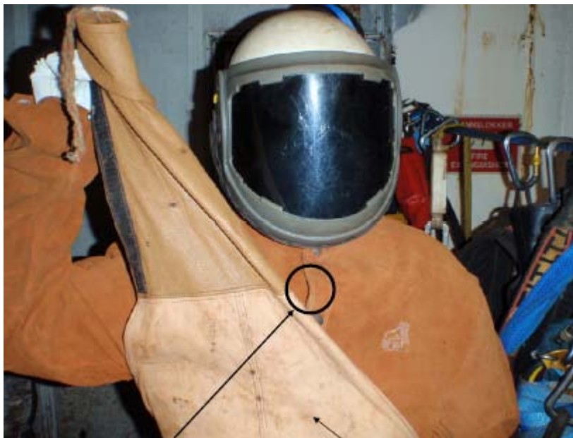
Figure 1 - Protective clothing for rope access technicians showing small opening through which hot particle passed
