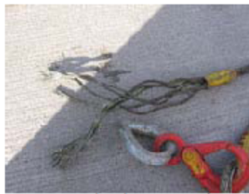
The crane pennant and the Flemish eye tails which have unravelled and pulled out of the ferrule
