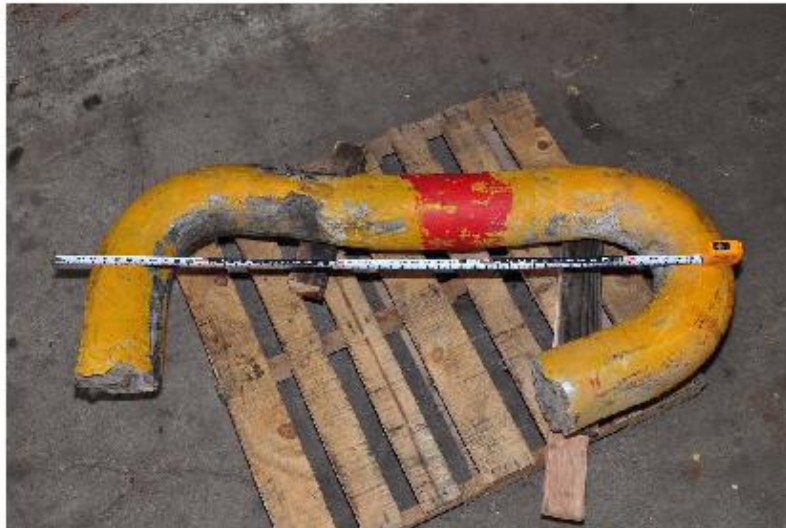
Failed Chain Link
