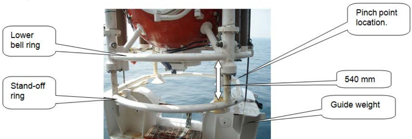
A view of dive bell showing pinch point location
