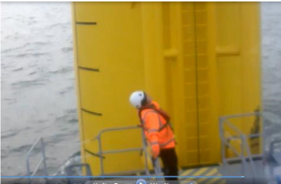
The crewman holds onto the handrail whilst the Master slowly repositions the vessel back into the boat landing; he shouts up to the technicians to STOP transfer until he tells them otherwise. Note: the vessel is now not centrally on the boat landing
