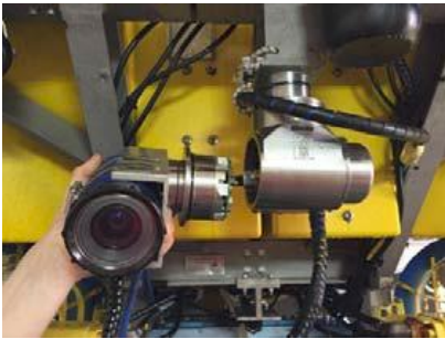
Close up of pan and tilt unit
