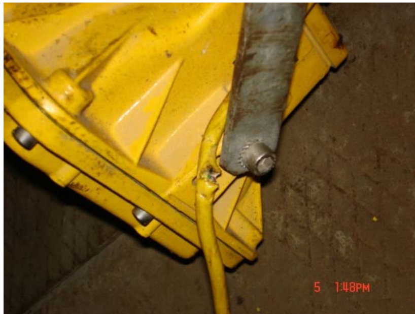
Damaged electrical cord
