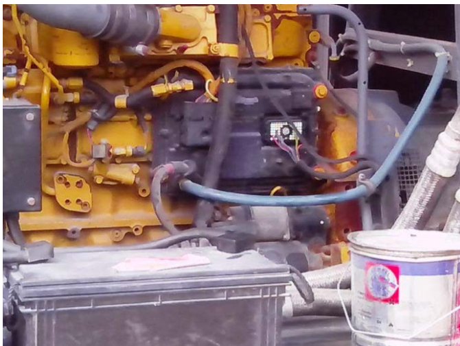
Figures: Compressor unit with PPE and flammable materials inappropriately stored inside
