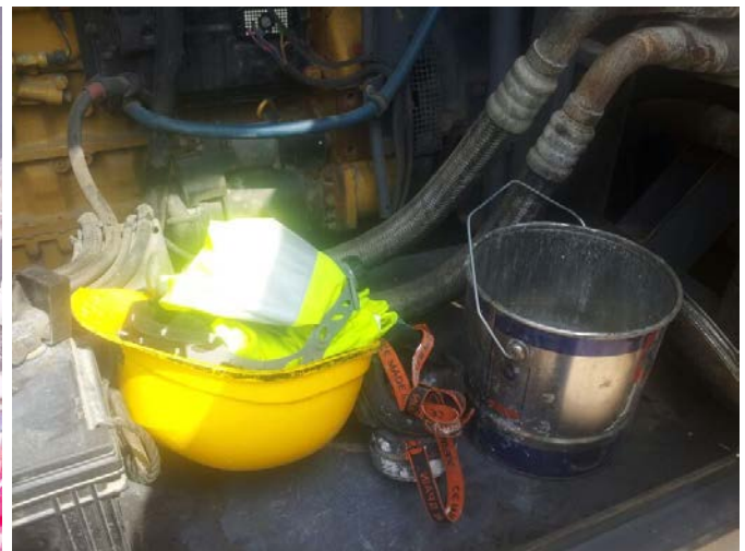
Figures: Compressor unit with PPE and flammable materials inappropriately stored inside
