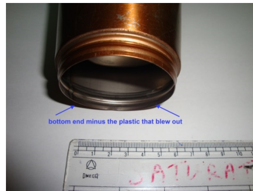
Figures: Showing thermos cup after explosion
