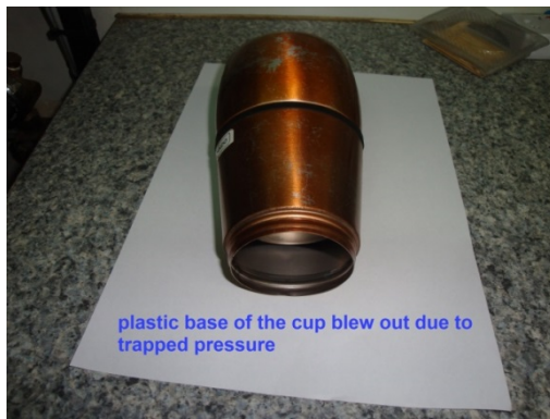
Figures: Showing thermos cup after explosion
