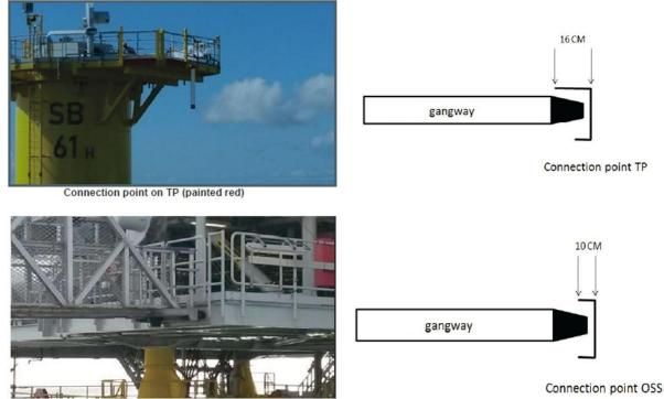
Connection point OSS (regular construction beam)
