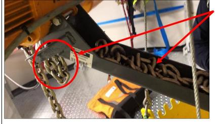
Example photograph showing how chain can kink causing it to back feed from feed tray due to the bucket being overfilled with chain
