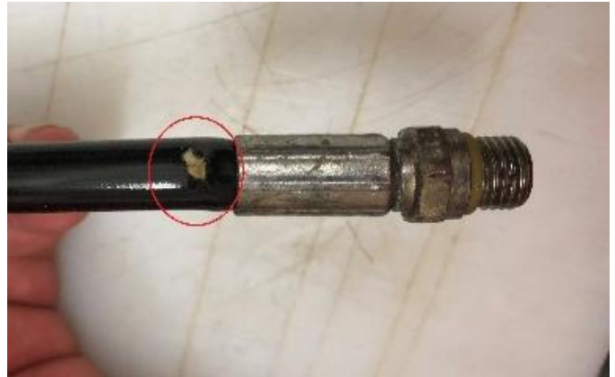
Damaged hose showed a damaged outer skin near the ferrule
