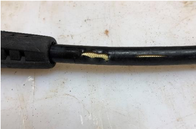
Damaged hose showed cuts in outer skin
