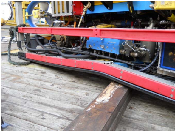
Figure 3: Damage to ROV frame
