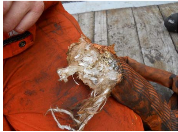
Figure 4: Sling after failure
