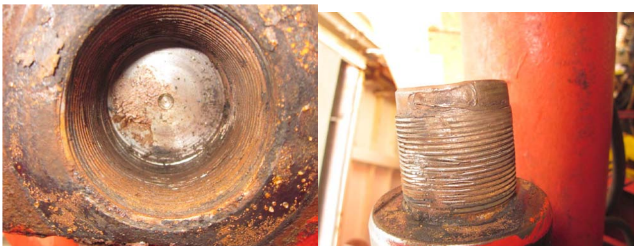
Figure: showing stripping out of threads
