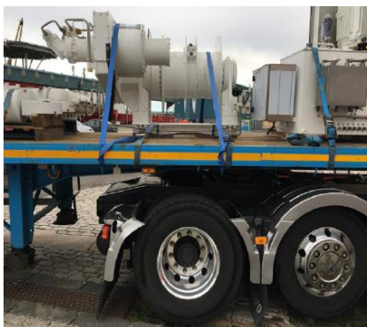
The winch after the incident – shown here correctly secured with ratchet straps
