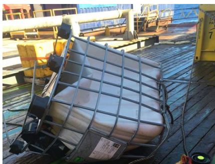
Result of dropped object – IBC after loss of load
