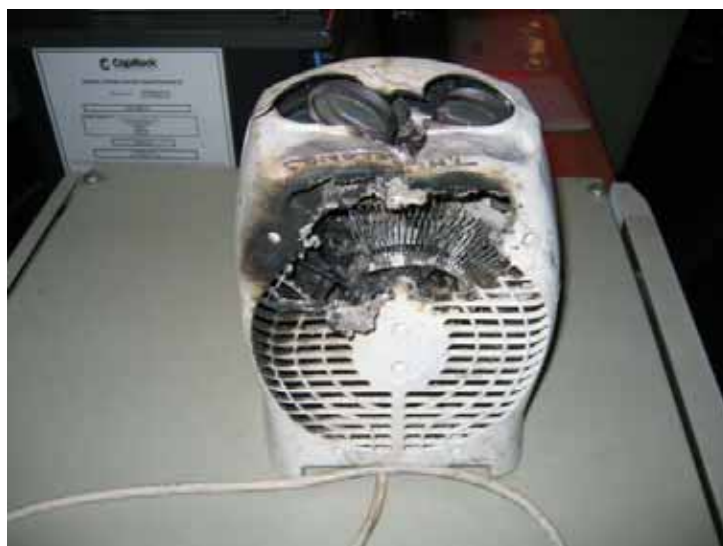
Damaged fan heater following fire
