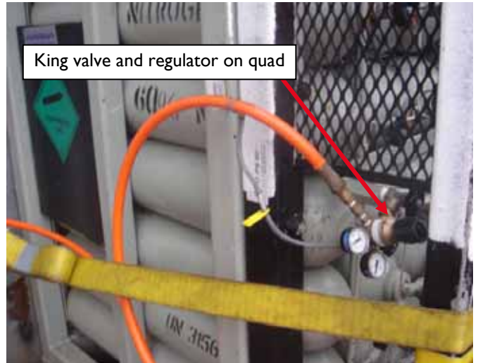
HP charging hose from supply quad used for decanting
