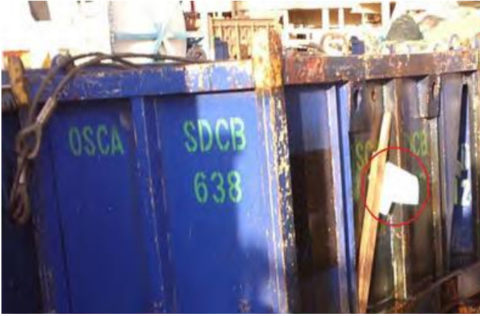
Showing punctured area of the DCB (circled)
