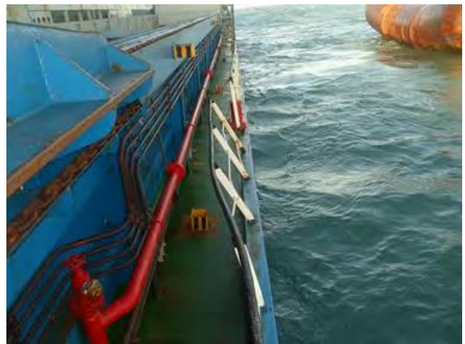
Showing the damage to the hand rails of the barge
