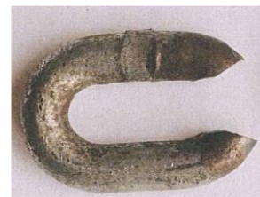
Link after break load testing
