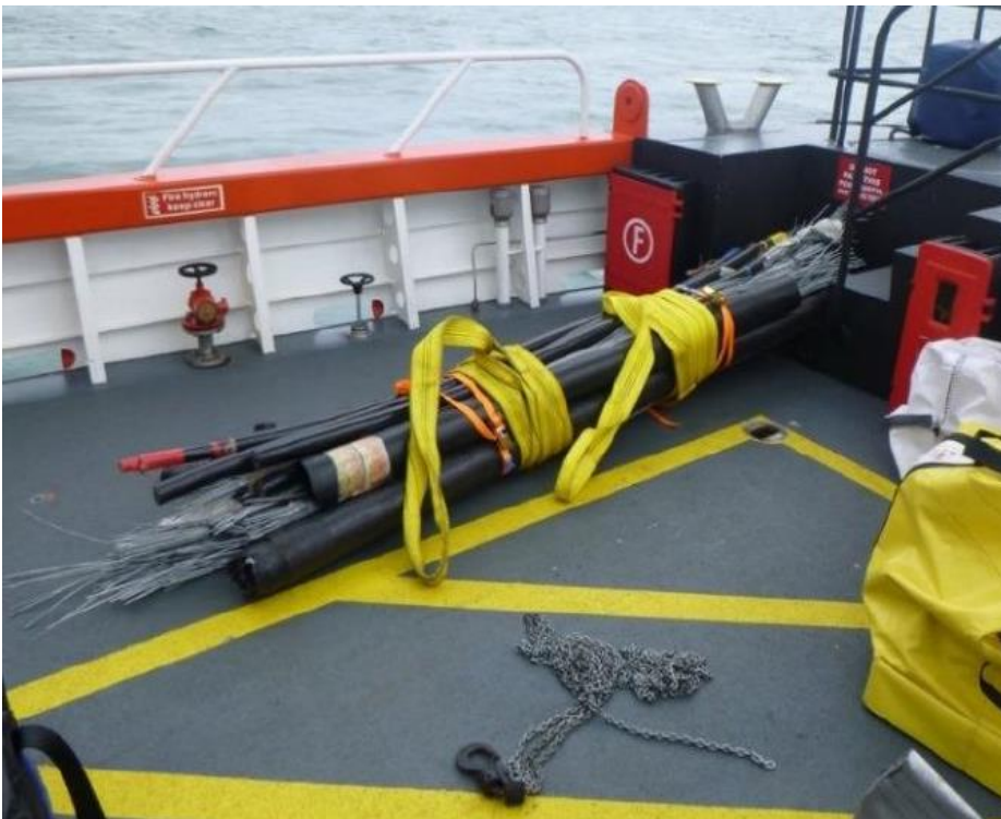
Dropped load and failed chain
