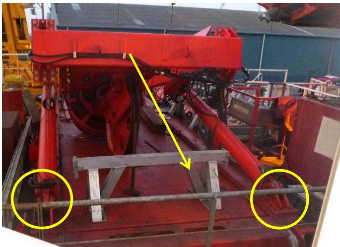
'A' frame in final position after collapse – showing where bolts were removed from feet of hydraulic rams
