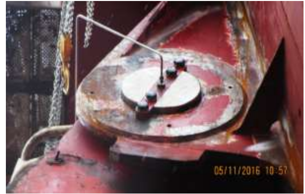
Renewed locking key anti rotation bolts and greasing line
