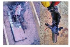
The incident highlights the importance of protecting equipment from water ingress, along with the importance of ensuring that care is taken whenever equipment is being dried out following exposure to water.
