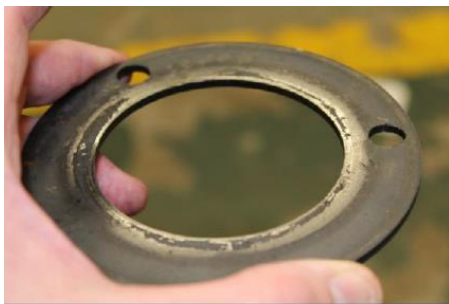
Hoist clutch plate (overload device) showing extensive corrosion on friction bearing surfaces.
