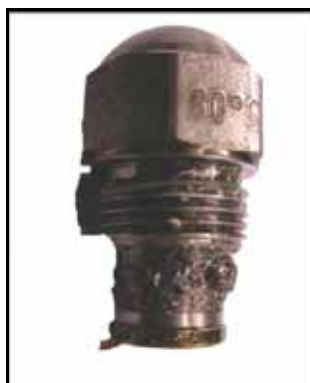
Blocked oil spray nozzle
