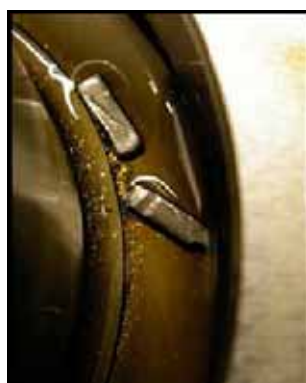
Broken check valve
