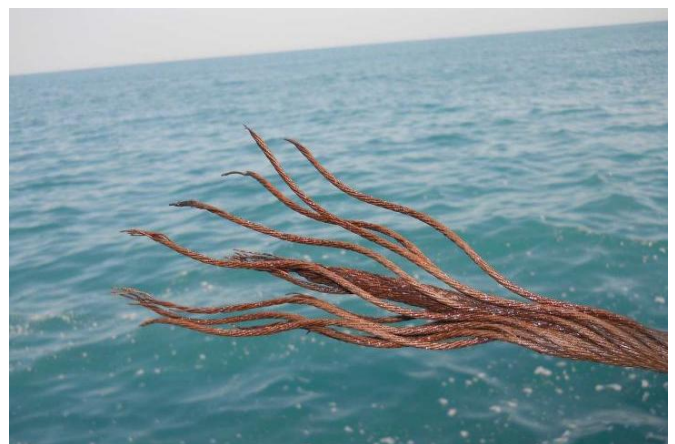
Parted winch wire
