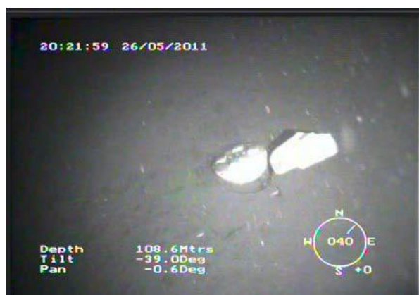
Clump weights landed on seabed
