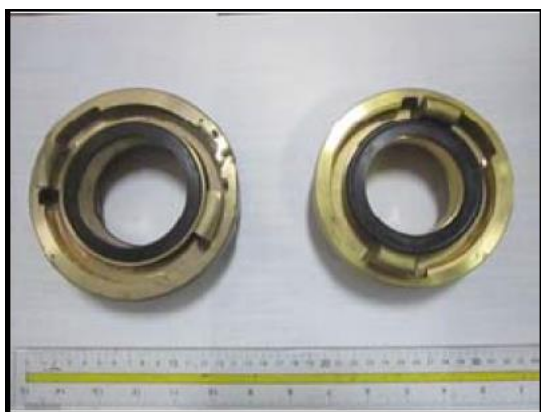
65mm hose coupling on right and 80mm hydrant coupling on left
