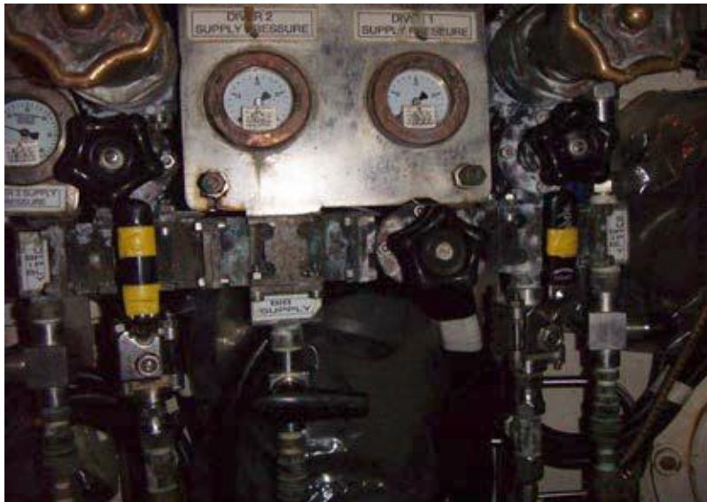
Dive bell panel showing modifications to the valve handles
