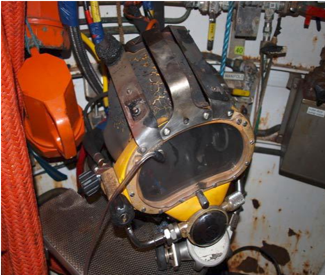
Damaged Kirby Morgan I7B helmet
