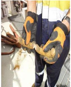
• Inspector checked lower links of the chain only and did not inspect the section hidden by the protective cover. The Inspector assumed that he had inspected sufficient percentage of the chain from which to infer the condition of the entire length. Chain under protective cover had significant corrosion.
