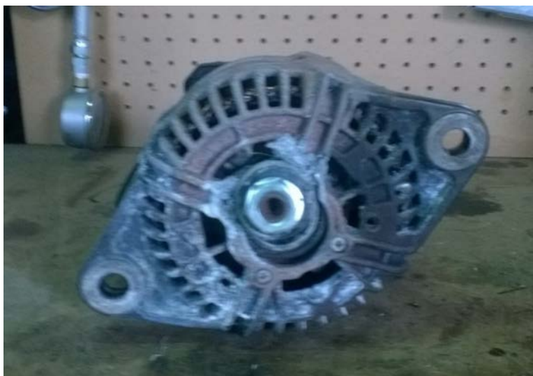
Figure: showing damaged alternator with shaft out of alignment due to bearing collapse
