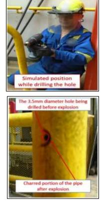
• The design of the handrail, using/creating hollow and enclosed structures, led to the conditions for accumulation of hazardous gas. There were no design features to allow for venting. The construction of the
