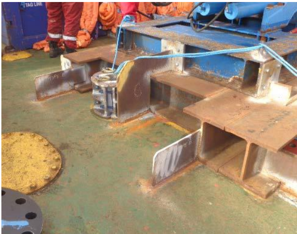
Figure: person tripped over Sea Fastening on right and banged his face on Sea Fastening on left resulting in a cut upper lip
