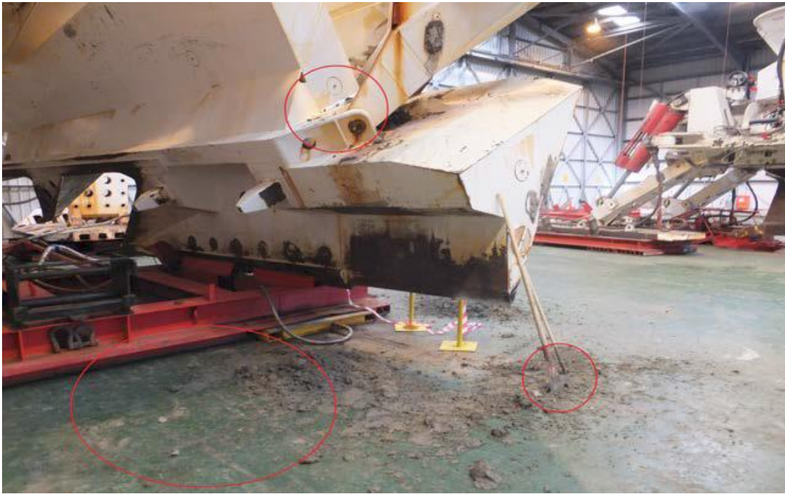
Figure: here, the injured person was working between the ground level as well as the air skate frame (20cm high); he stepped down and slipped on the silt in the bottom of the dry dock during cleaning operations, and fell to the floor banging his head, he also cut his face and bruised his ribs and hip. Red circles indicate area being cleaned; area where injured person fell, and tools being used.
