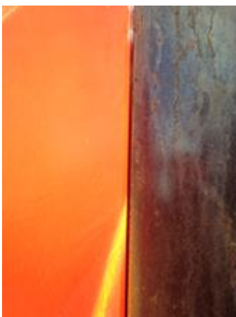
Figures: showing varying distance between winch drum and guards
