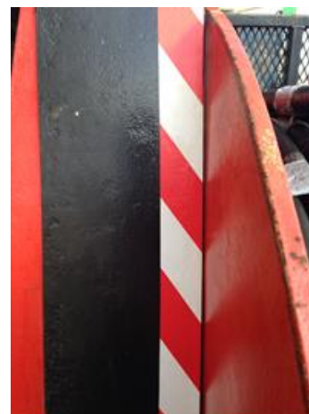
Figure: added strip of additional guarding and safety tape to highlight potential 'pinch' points to operators.
