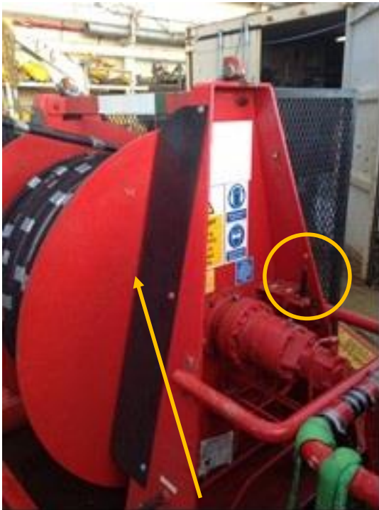
Figure: hydraulic winch showing control lever and the guard in which the operator trapped his thumb
