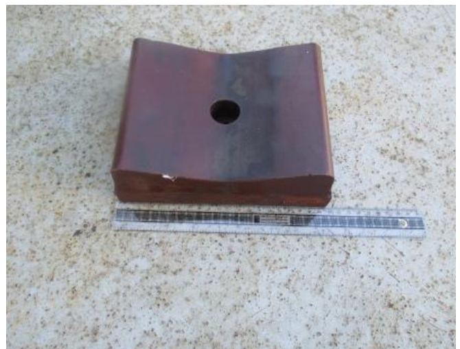
Figure: tensioner pad (weight 7kg)
