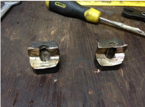
Figure: material loss on the bronze bushing
