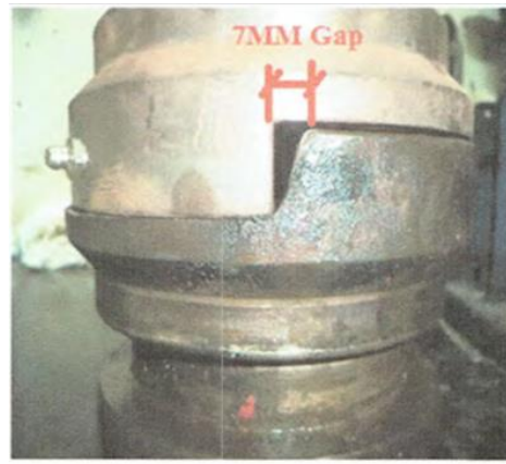
Figure: clutch cog wear showing \frac{1}{2} the actual gap against the replacement clutch.
