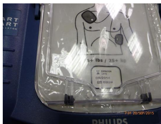
The pads on the AED were out of date;
