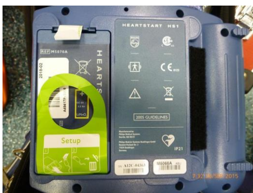
The battery had been removed or had been fitted incorrectly to the device. This was contrary to advice in the user manual for the item.
