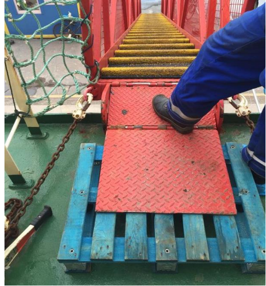
Here an employee stepped on the hinge of the gangway access ramp when it buckled.
