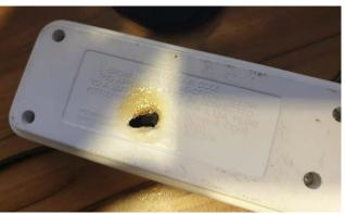
Vessels use residual current devices (RCDs). These devices effectively need to see balance on each phase and in the instance of a short on either phase, will trip the breaker/RCD. When the extension lead was connected to the ships power supply, the varistors heated up until one of the phases saw more or less current, thus tripping the breaker/RCD.
