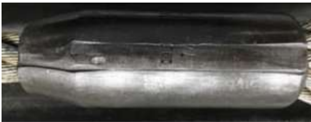
Correctly pressed 20mm steel ferrule
