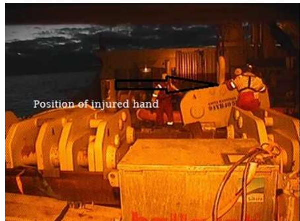
H-link started swinging when being lowered into sled
