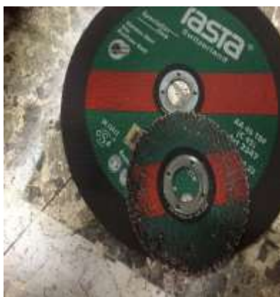
Worn disc and as new disc
