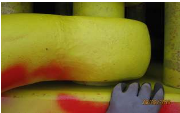
Showing gap between shackle body and H-link
