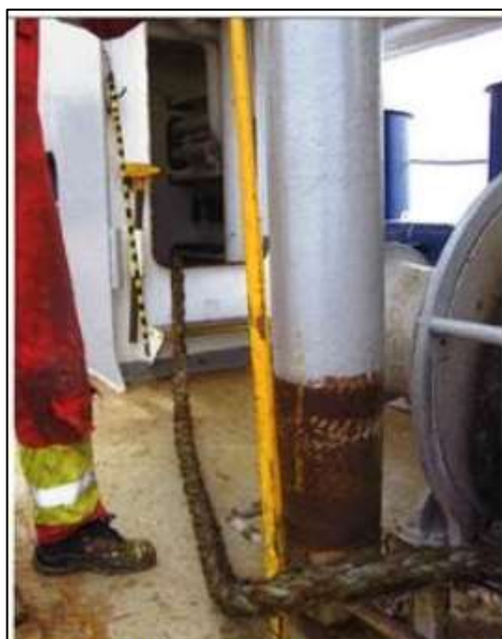
Side view showing spooling direction of mooring line.
