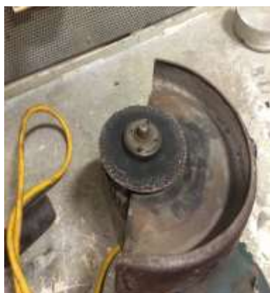
9” Grinder with heavily worn disc attached
