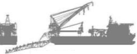
Pipelay vessel – rigid
