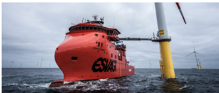
A service operation vessel (SOV) on DP alongside a turbine, with its walk to work gangway deployed.
