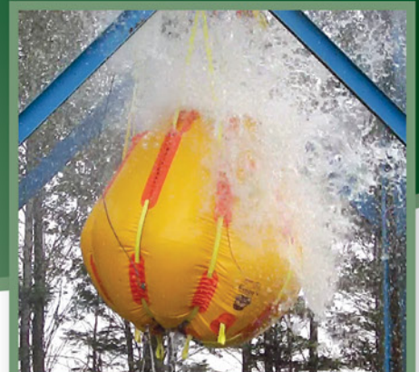
5 tonnes parachute air lift bag, before and during type testing. Recorded peak load of 51 tonnes, giving 10:1 safety factor.
