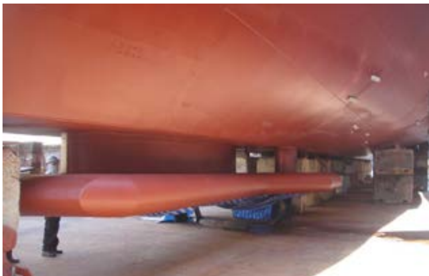
Fugro collects multibeam echosounder data from specialist equipment housed in a gondola platform mounted beneath the hull of survey vessel Fugro Equator
