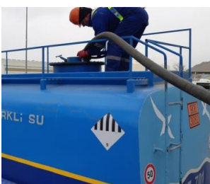
Incorrect connection practices – hose hung through the tank hatch
