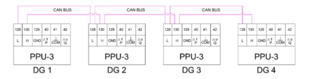
Further tests demonstrated that switching the power supply of DG2 PPU on and off would cause the screens of other PPUs to flash and reboot. This was observed to occur approximately fifty percent of the time. The flashing and reboot would cause the respective generator breaker to trip. It was noted that cycling the power of DG2 PPU could cause any other generator to trip, regardless of redundant group.
