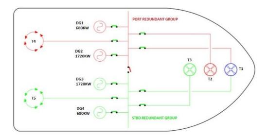
The vessel is designed to operate with open bus ties at all power levels. At the time of the incident, the main bus tie was open, separating the two redundant groups. All generators were online. The weather was fair and sea conditions were light with wind speed of 1 knot, current 2 knots and wave height of 1m.
