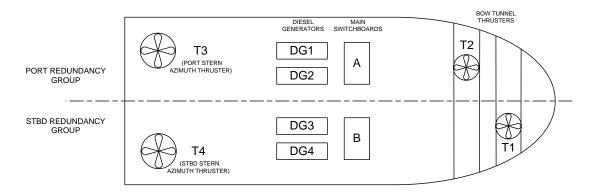
The bus ties between the redundant groups were closed creating a common power and propulsion system and DG1, 2 & 3 were online, DG4 on standby. The weather was typical for the area: wind speed 4kts, current 3.0kts and wave height 1.5m.
