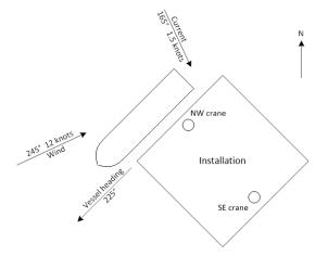
The port aft azimuth developed a failure that led to it tripping out of DP control and its main circuit breaker opened. As the vessel was being operated within its environmental envelope and the thruster failure did not exceed the designed worst case failure, the vessel maintained position.
