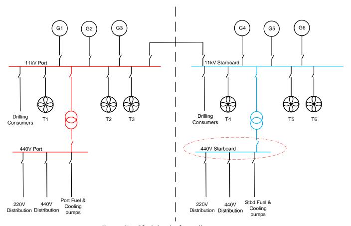
Figure: Simplified sketch of vessel's power system
