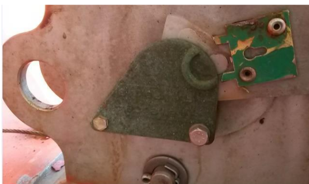
The misaligned forward hook with 'padlock symbol'.
