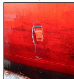
Divers magnet used to minimize spill
