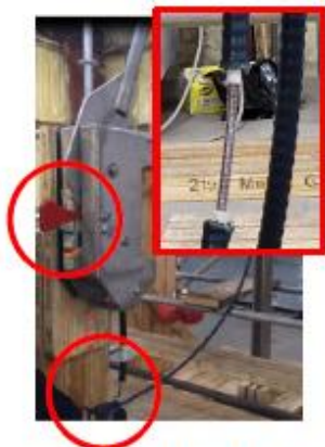
Image 2: Forces cause the outer layers of the cable to separate. The release handle stays closed.
