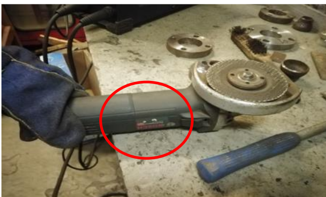
Selector switch grinder (not permitted)
