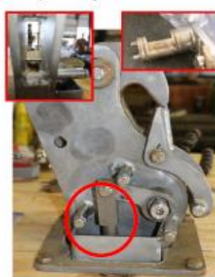
Image 3: At the hook end, the cable end rod moves. This causes the locking shaft to rotate.
