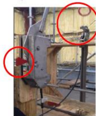
Image 4: If the locking shaft turns enough, the hook will release, even as the release handle stays locked.
